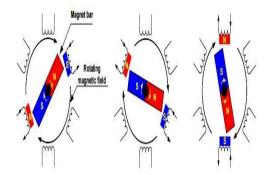
As the rotor nears coil A, coil B is energized. As the rotor nears coil B, coil C is energized.
